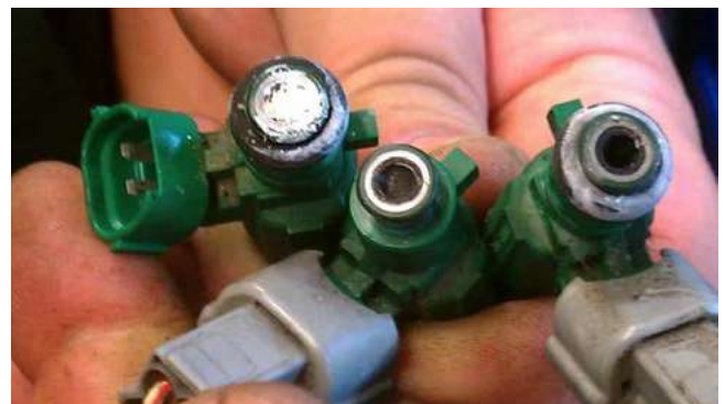
Corrosion in fuel injector caused by EBP
